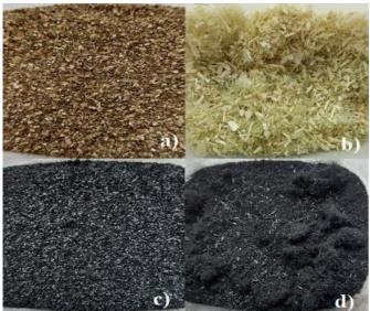
Fig. 1. **Primary raw material and biochar for fibre hemp:** a – seed husk; b – stem; c – seed husk biochar; d – stem biochar
